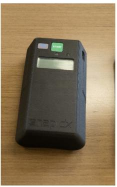
2. Press and hold Wi-Fi (I) and start button (E) together for 2 seconds and release when blue light turns on (K)
