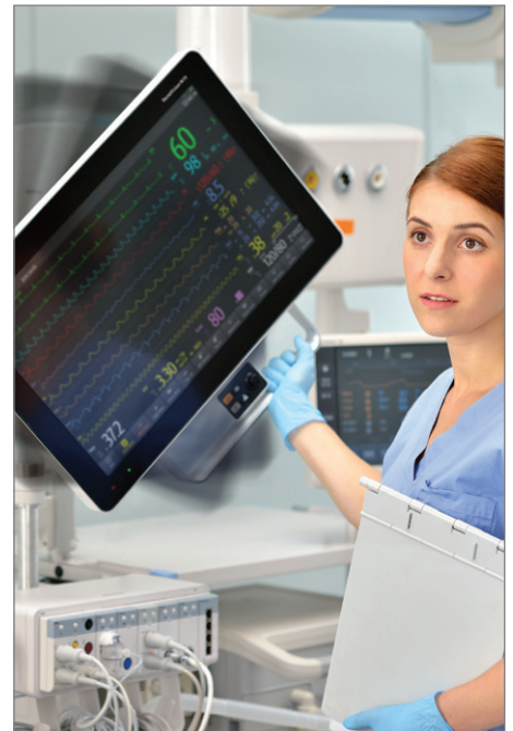
Choose portrait orientation for maximum number of waveforms or landscape orientation for longer waveforms.
