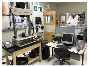
The axial/torsional configuration of the Bionix tabletop system enables biaxial testing, controlling torsional moments up to  $\pm 100$  N m and total rotations of 270°. It is excellent for testing the durability and wear properties of components such as knee, hip and spine implants. When paired with specialized subsystems and accessories, it is capable of performing both simple and complex kinematics studies of skeletal tissue and orthopaedic constructs.
