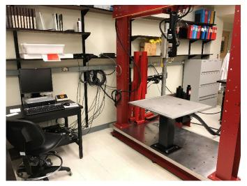
Currently MTS\_1 & MTS\_2 both have two actuators that are configured in a horizontal and vertical orientation. However either system can borrow the other two actuators and configure them to best suit a four actuator test.
