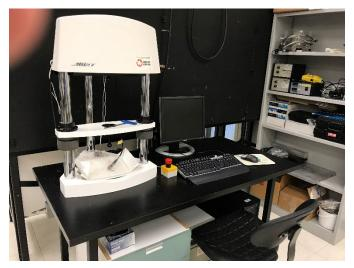
The ElectroForce 3220 test instruments feature a 225 N maximum force. With the versatility of static to 300 Hz frequency response, the tabletop configuration is adaptable to a variety of biomedical research and engineered materials test applications, creep under dynamic loading, fatigue, stress relaxation and special environments (water bath). Technical Specifications:
